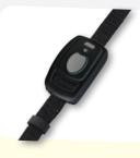
Falls detector This device raises an alarm in the monitoring centre automatically, when movement and impact associated with a fall is detected.
